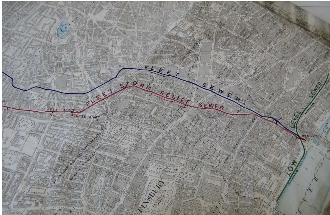
Figure 2: Map Showing Position and Dimensions of Fleet Sewer and Storm Relief Sewer at Holborn, LCC Drainage Committee, 1905
